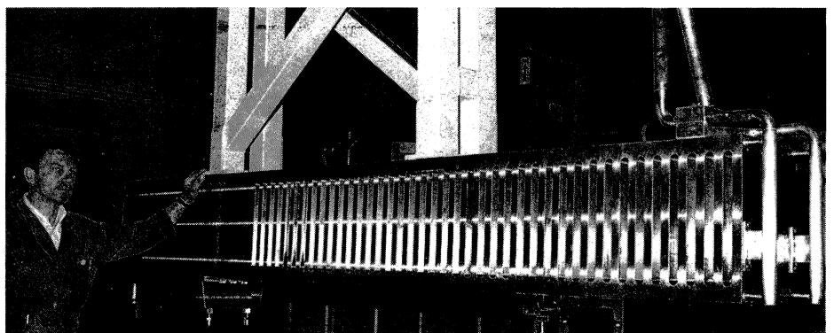
A 'beam dump' such as this is designed to produce a residual secondary beam which can be examined for signs of new particles. Most of the secondary particles produced when the primary proton beam hits the end of the dump are absorbed along the length of the target.
